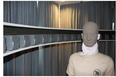
Figure 4.7: Recording of HRTFs with FABIAN in room Pinta . Note that this picture is from a recording session where FABIAN was placed out of the center and did not wear headphones.
